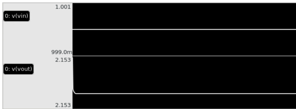
Figure 5.12: Resulting waveform for a transimpedance amplifier
